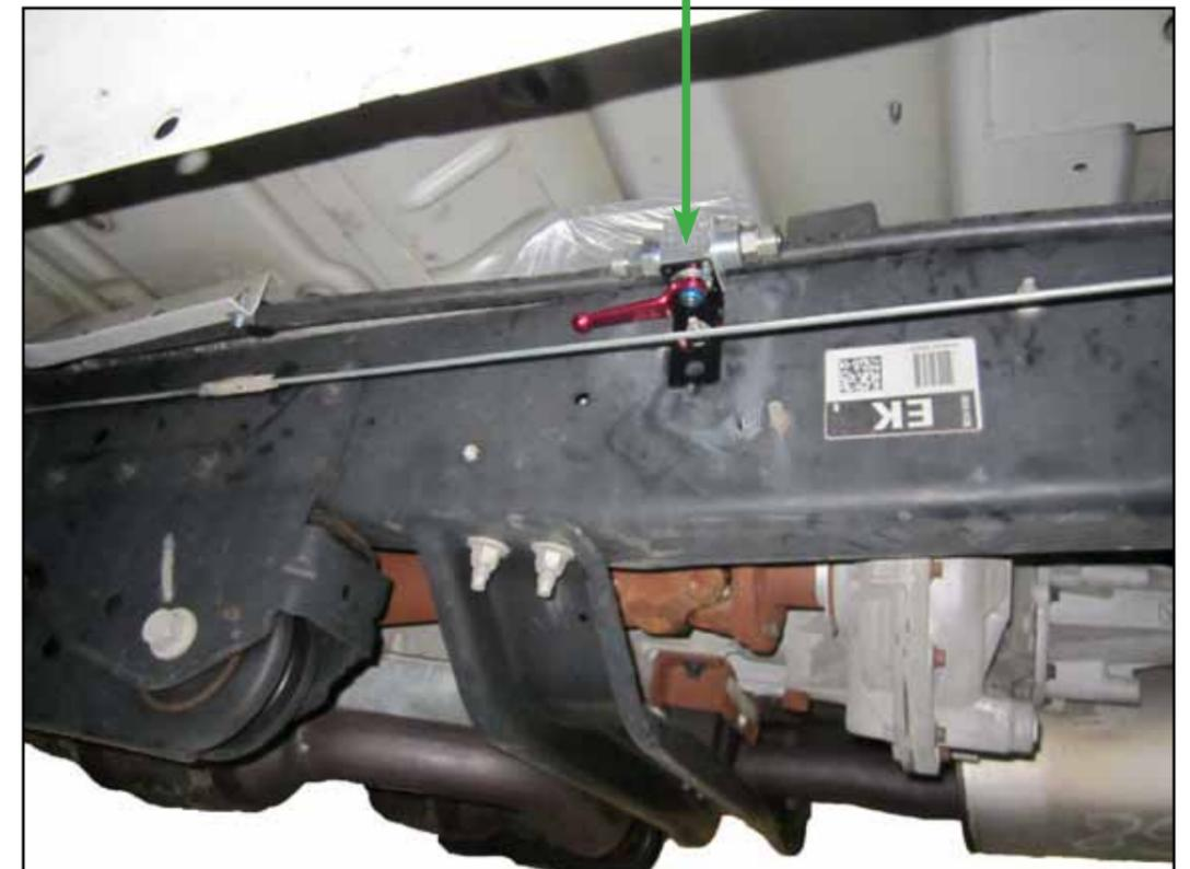
1. Install valve assembly. Secure with OEM nut and tighten to 45 ft-lbs.
